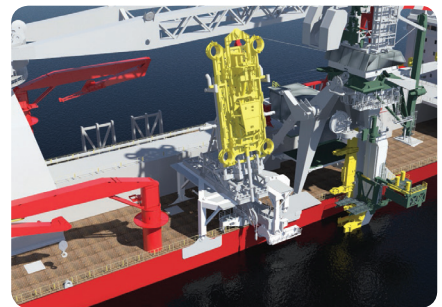
24" PLET installation from Seven Borealis – 3D
